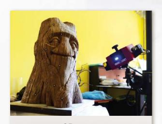
3D scan: maps the real object using a 3D scanner and transfer it to 3D models on computer
